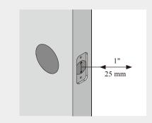
Measure to confirm that the door is 1-3/8" D to 2" (35 mm or 50 mm)thick .
