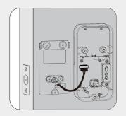
D Secure the interior assembly with the supplied screws.
