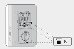
B Rotate the turnpiece in vertical position and make sure the latch is still fully retracted (in the unlocked position). Insert the torque blade through the center hole in the mounting plate.
