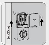
C Test the turnpiece for smooth rotation. If turnpiece doesn't rotate, repeat step 4C, making sure the turnpiece in vertical position.
