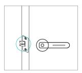
2) Use 2 wood screws to secure latch.
