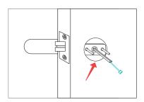
5) Press slightly on the battery cover and remove the screw on the battery panel. Open the battery cover.
