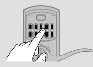
Make sure the door is open. **If you have not enabled a Programming Code,** press and release the Program button. You will hear two beeps.
