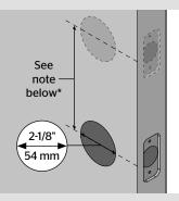
\*If you are installing this lever below an existing lock or you plan to install a lock above this lever, make sure that the distance between holes is at least 6-1/2" (165 mm).
