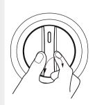
Rotate the thumb turn to Unlock position.
