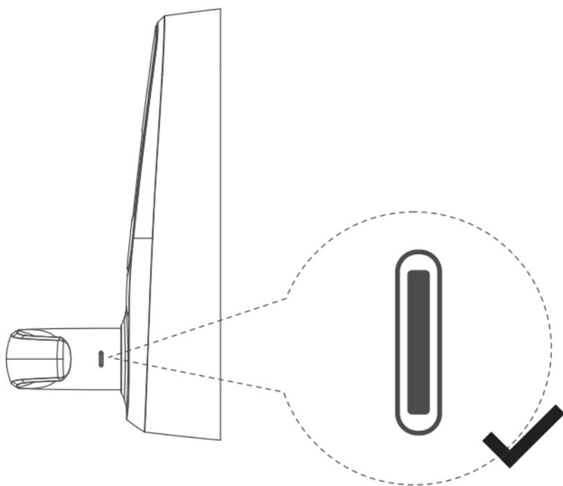
The handle is plugged in correctly.
