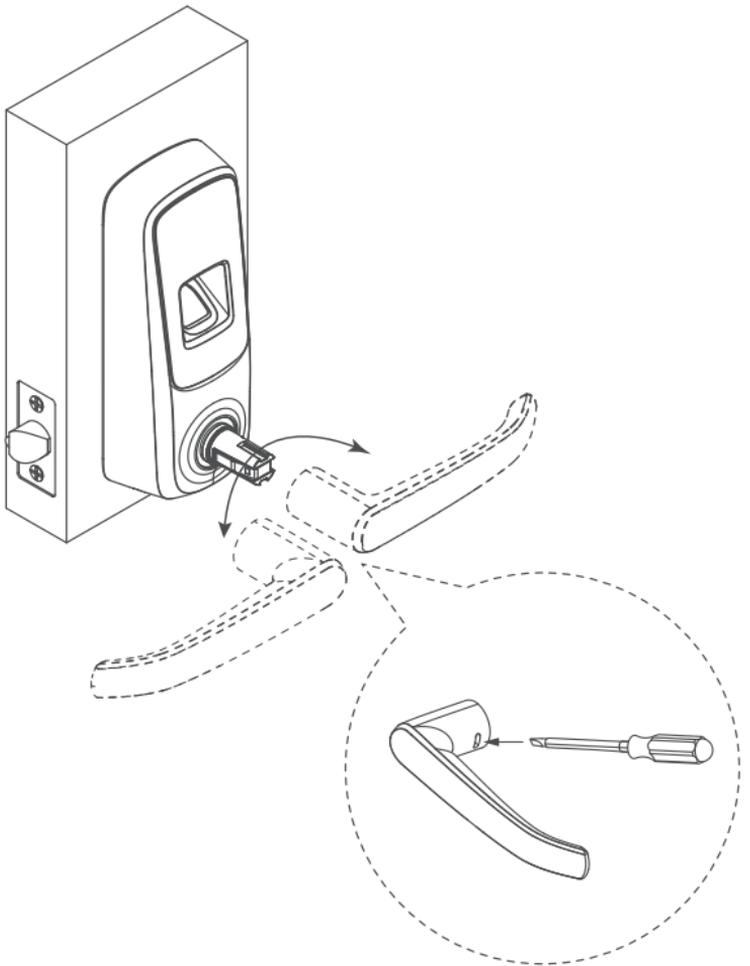
If the handles are installed in the wrong direction, you need to remove them and re-install.
